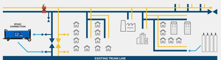
7) To inert the pipe prior to cut and cap, continue to run ZEVAC while injecting nitrogen at far end(s) until gas mix is below LEL.
